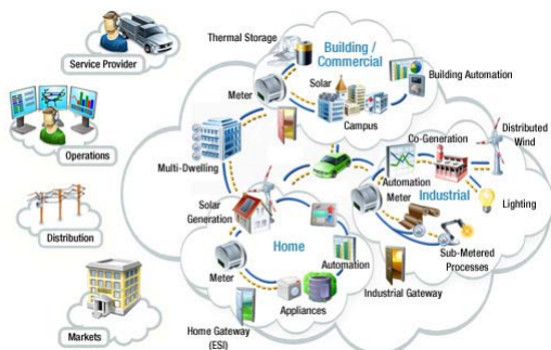
Figure 4. Smart Grid Cyber Security Conceptual Model - NIST Smart Grid Framework - Customer
